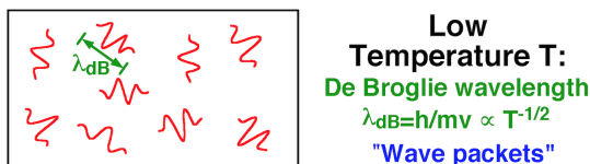
FIGURE 2. Simplified quantum description of gas at low temperature, in which the particles are regarded as wave packets with a spatial extent of the order of the de Broglie wavelength, \lambda_{dB} .
